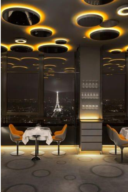
Figure 5-11; LED tape lights around false ceiling patterns. Source: pinterest.com
