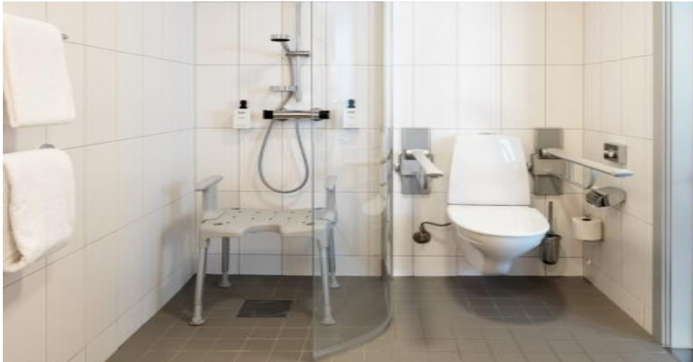
Figure 2.13: Universally designed bathroom, 2019. (Source: www.zeroproject.org , 2019).
